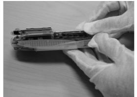
Note: Make sure that the LCD assembly is completely loose from the D-cover snaps to minimize the risk of bending the LCD board.
