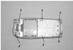
Remove the six screws using a nonconductive screwdriver (Presicion Torx Driver T6 Required).
