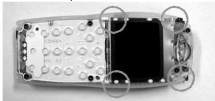
Insert a nonconductive tool on the side of the LCD (four snaps circled above) and carefully snap the LCD assembly out from the D-cover.
