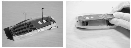
The PWB (shown at left) can be removed by lifting it up from the guide pins in the D-cover.
